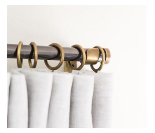
Extended End Bracket Brackets over 4" projection are considered an Extended Bracket and are fabricated using 3/16" flatbar. Typically used in applications with very heavy drapery panels or where you need to extend past a sheer or a shade Shown: HDB-X-6-125 (Heavy Duty Bracket - Extended Bracket - 6" projection - for 1.25" Diameter Rod)
